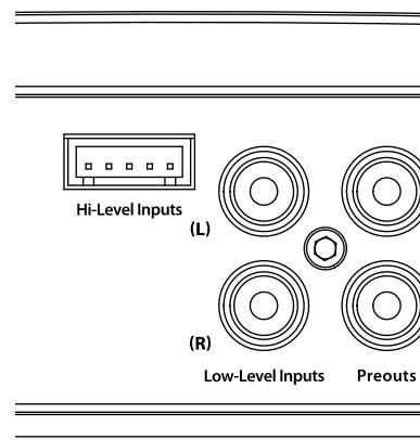
You may run a stereo or a mono signal into the inputs of the amplifier. The amplifier's input section automatically sums stereo signals to mono for the internal amplifier section.
