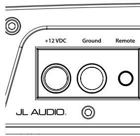
The amplifier's "+12 VDC" (positive) and "Ground" (ground) connections are designed to accept up to 4 AWG power wire.
