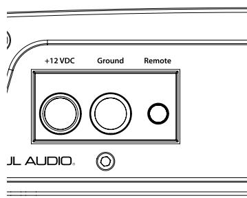
The amplifier will turn on when +12V is present at its “**Remote**” input and turn off when +12V is switched off. If a source unit does not have a dedicated remote turn-on output, the amplifier's turn-on lead can be connected to +12V via a switch that derives power from an ignition-switched circuit.
